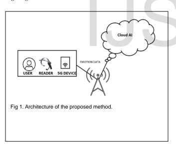
The clienct side comprises of the user, brainwave reader, which can be embedded as a chip to user and a 5G smart device or kiosk to which the reader is connected. The data is collected from user continuously and is transmitted to cloud.
